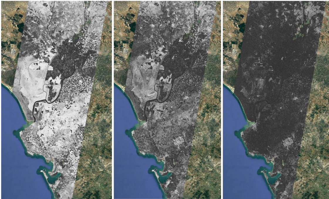
Figure 8 SINCOHMAP Project: Interferometric coherence evolution considering consecutive interferometric pairs of 6, 12 and 18 days. Sentinel-1 A/B data over Doñana (Spain)
