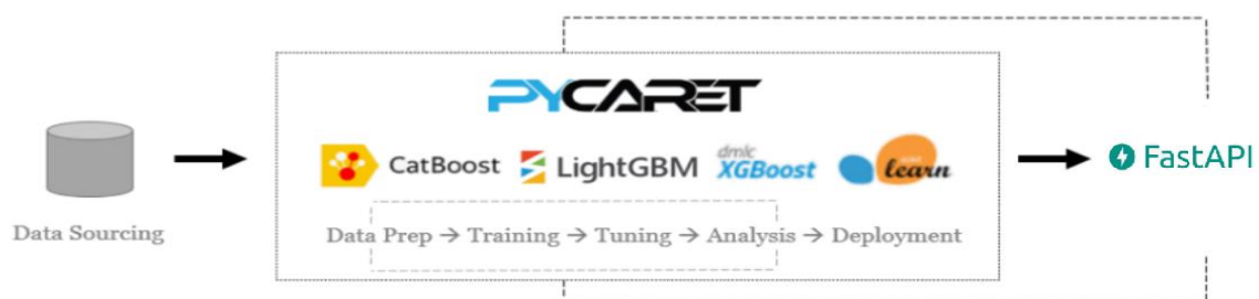
Figure 68: Using PYCAREt and web frameworks for building APIs with Python like FastAPI makes it possible to generate machine learning pipelines for batch or real-time predictions.
